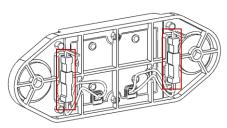
Connect the male and female connectors and ensure they are securely clipped together.
