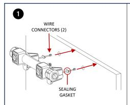
Insert both wire connectors into the holes of the shield.
